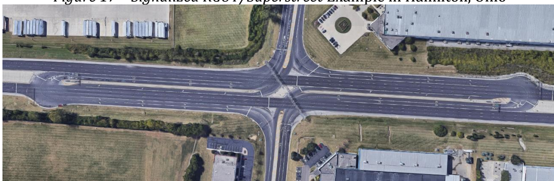
Figure 17 – Signalized RCUT/Superstreet Example in Hamilton, Ohio
